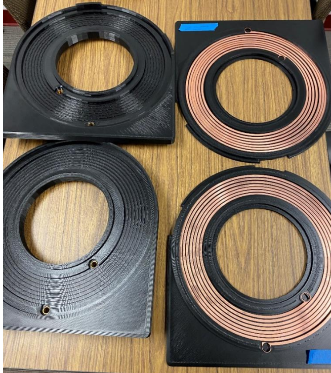
Copper spirals machined for the hot water-based heating system assembly – FIX project.
