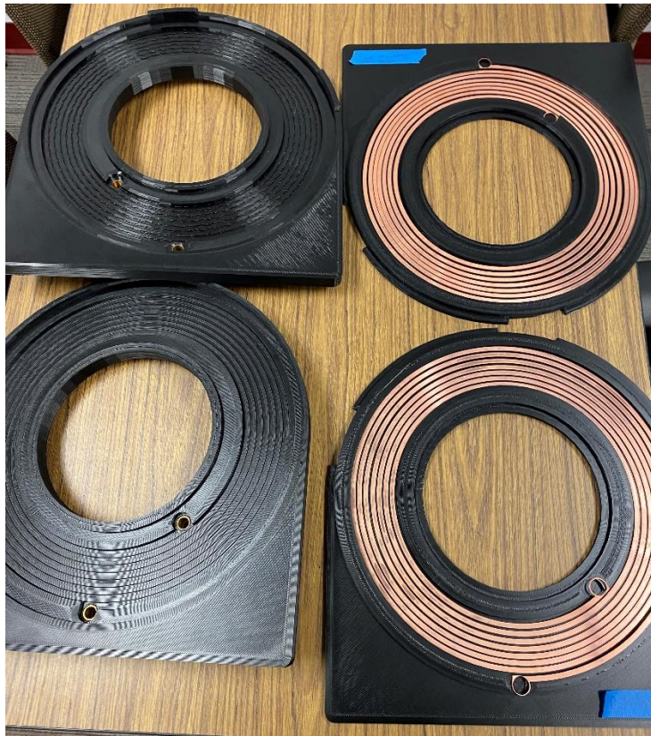
Copper spirals machined for Hot Water Based Heating System Assembly – FIX project.
