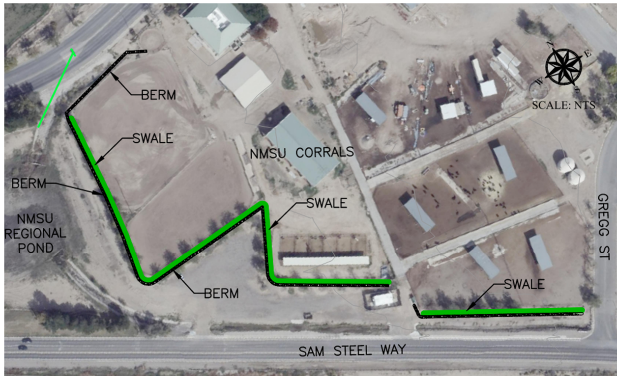
FIGURE 8-16: CORRALS RUNOFF MITIGATION – PLAN
